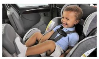
A rear-facing car seat supports the entire head, neck, and back of a child and the shell of the car seat absorbs the force of a crash. When a child sits in a rear-facing car seat, the head moves with the seat, reducing the risk of injuries to a child's head, neck, and spine.
